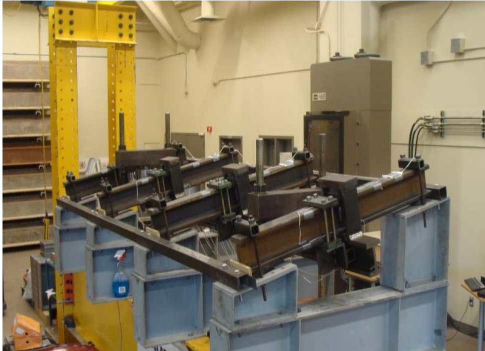
Figure 3 – Instrumented Specimen Mounted on the Specially Designed Test Frame
