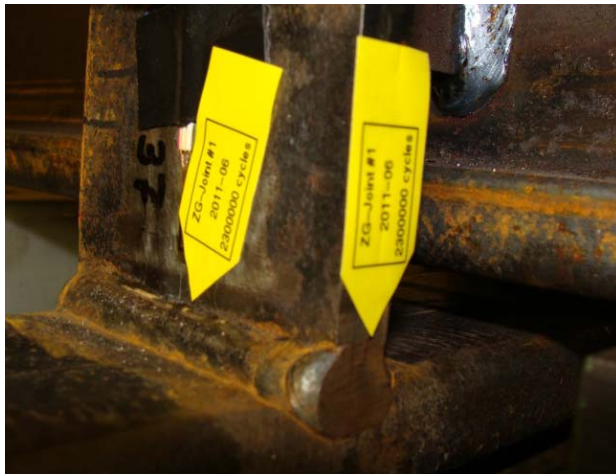
Figure 6 – Type B Cracking at Stirrup S2 at 2 300 000 and 2 927 965 cycles
